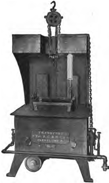
Fig. 191. Typical Tempering Furnace Courtesy of Strong, Carlisle and Hammond Company, Cleveland, Ohio
